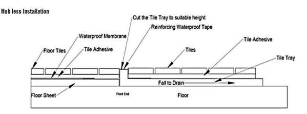
The waterproof membrane should extend at least 1500mm from centre of the tile tray outlet. The fall of the floor outside the tile tray must be towards the tile tray outlet to comply with local standards.
